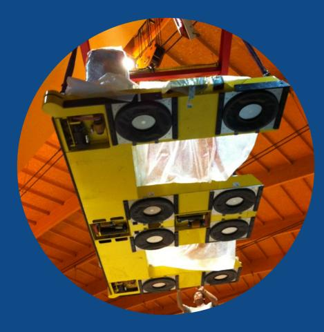
Air Casters are also often called Air Cushions, Air Skates or even Air Bearings. They can be mounted permanently underneath specific equipment or tools or used as a modular air caster system.
